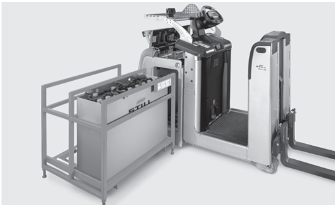
Always available thanks to lateral battery change
