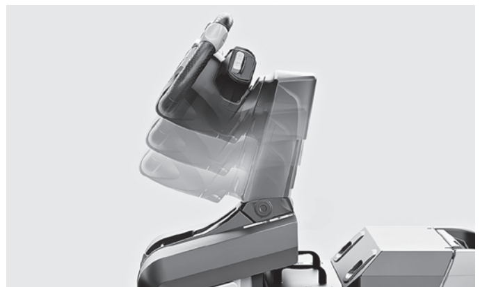
Optimal ergonomics owing to the height-adjustable steering wheel at a slight angle for individual operator preferences
